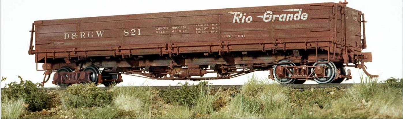
The "S" Scale Narrow Gauge "Drop Bottom Gondola" car above exemplifies the "Scratch Brush Weathering" technique. More photos of this and other contest quality models can be seen on our web site at [www.p-b-l.com](http://www.p-b-l.com). (Click on "Rolling Stock.") STAR BRAND PAINTS lend themselves nicely to this technique because they are fast drying.
